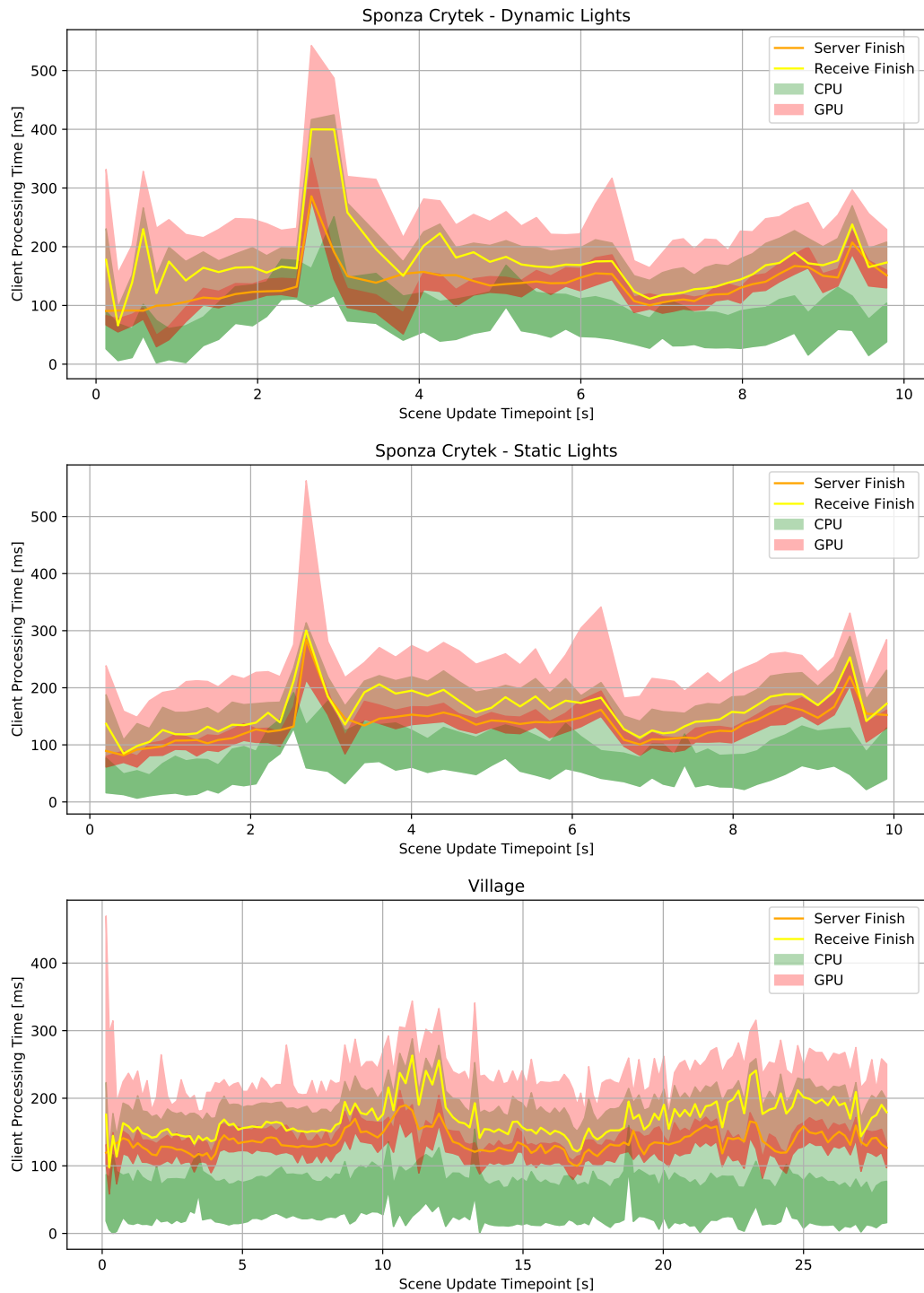
Figure 7.3: Client scene updating times. Vertical axis represents timeline per scene update at given timepoint at horizontal axis. Green / red areas shows time ranges of processing CPU / GPU tasks. Darker areas shows real time spent processing tasks (parallel on CPU serial on GPU) and brighter areas shows idle time or waiting for dependency, e.g., data from the server or GPU task for CPU task. Lighter GPU area also contains time spent on rendering of the current scene, as GPU tasks and scene rendering is interlaced.
