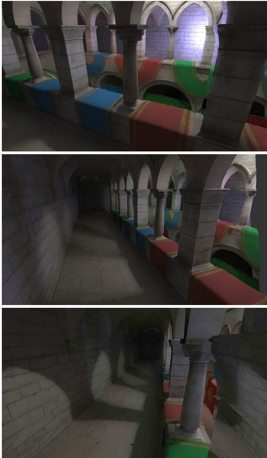
Figure 7.9: Sponza Crytek scene with dynamic lights (top and middle) and static lights (bottom) rendered on the client. Note: bottom has sharper shadows than middle, because denoise filter works better for static scenes.
