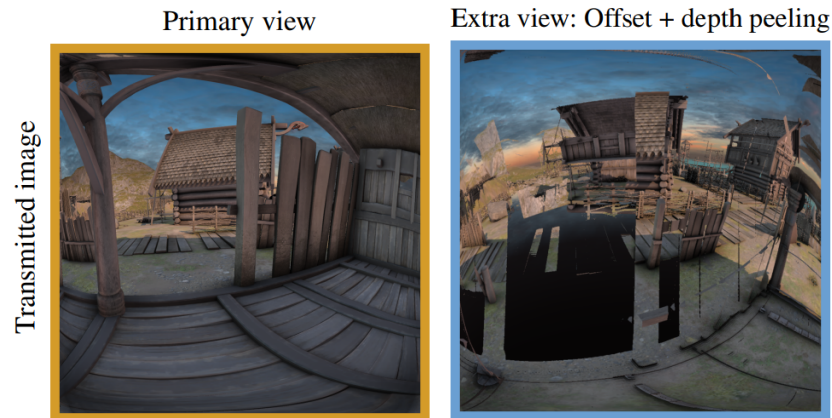
Figure 2.1: Proxy-guided Image-based Rendering for Mobile Devices: primary and extra view (source: [RKR + 16]).
